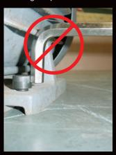
Stubby L-Wrenches eliminate the need to trim and file the short arm. A trimmed L-Wrench introduces burrs, and still does not have the tight radius of a dedicated Stubby wrench.
