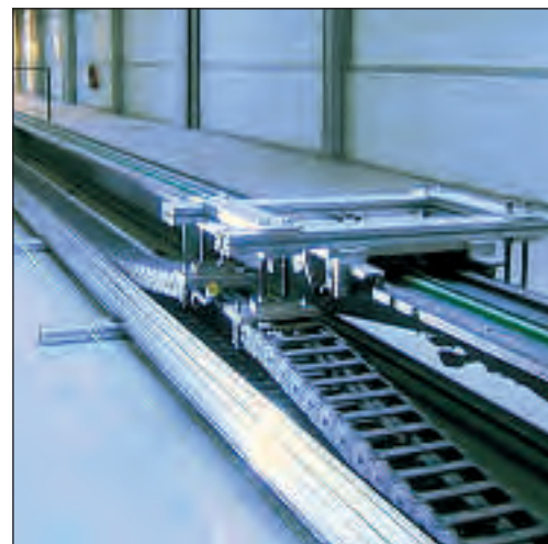
55 m endurance test unit for testing highly flexible power chain cables.
