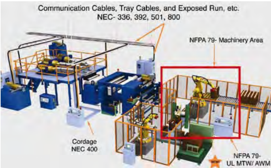
The diagram illustrates key NEC® and NFPA regulatory codes for an industrial plant manufacturing floor. Each code calls out permissible cables. 'NEC®' is a registered trademark of the National Fire Protection Association.
