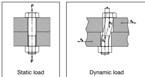
With **static loads** in axial direction, settling, which is dependent on the number and shape of the separation joints between the tensile building components, can lead to a complete loss of preload. With this kind of load, loss of preload may be counteracted with certain constructive measures or by using screw-settling locks.
