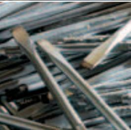
The uncoated tips are burnished in an automatic unit, the resulting dark colour giving the so-called "Black Point".
