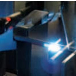
A laser system is then used to apply the screwdriver size and serial number. This means that even after they are sold, we can still identify exactly which raw materials were used to make PB tools.
