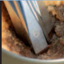
The finished blades are treated with a corrosion protection agent. Even the "Black Point" is protected against rust by this process.
