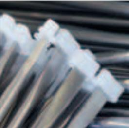
The tips are covered with special caps and remain uncoated during the plating process. This increases dimensional accuracy and helps the blade grip the screw slot.
