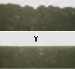
The surface is then prepared for galvanising by grinding.
