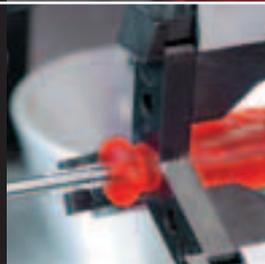
The labelling on the handle and blade is lined up and the two parts are brought together.
