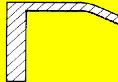
HASBERG Protective vice jaw sets made of light metal (plastic not available) have pressed retaining springs, so they remain firmly in place on any vice and do not fall off.
