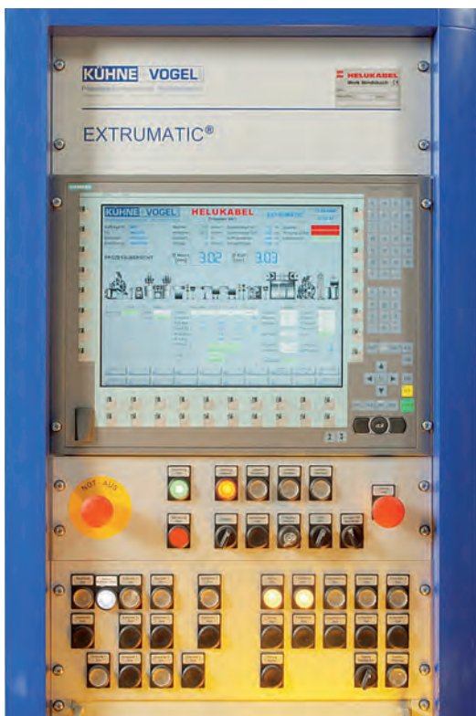
Standardised process control and visualisation of an extrusion system at our Windsbach factory.
