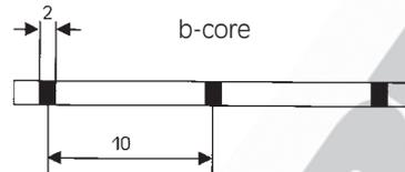
The colour identifications of the a- and b-cores of switchboard cables are coded with a basic colour and colour rings.
