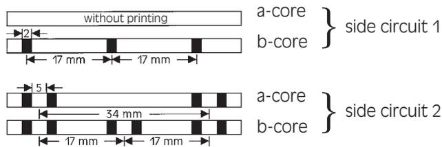
The cores of 5 star quads of a sub unit are counted according to the sequence of basic colours:
