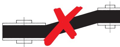
Axial misalignment of pulleys
