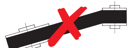
Horizontal angle deviation of the shafts
