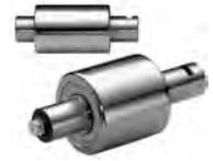
**Water-Cooled Split Bearings** are designed to handle extreme loads at elevated temperatures. The races are horizontally split and allow simple roller and race replacement without moving the equipment or rolls on which they are mounted. A classic application is a driven strand guide rollers on a continuous caster.
