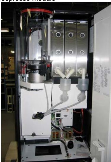
Boiler unit in the coffee machine ES 5100
